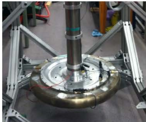
Fig. 3. Left – beam dump prototype for the mechanical testing; right – simulation results (lines) vs. the experimental data (dots). Blue – vertical, red – tangential flow velocities, averaged over the points having the same radius. The dashed line shows the tangential velocity when the wall surface roughness 0.1 mm is taken into account. (For interpretation of the references to colour in this figure legend, the reader is referred to the web version of this article.)
