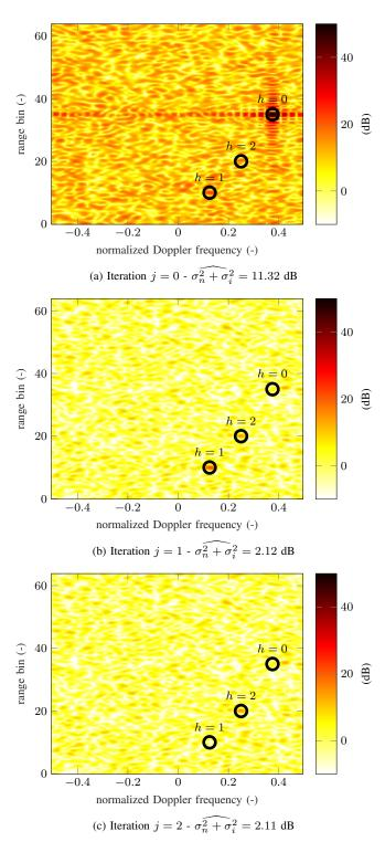
Fig. 5. Illustration of our CLEAN-based procedure on a range-Doppler map obtained from the radar scene in Table I. QPSK symbols such that  $\sigma_{d-1}^2=1$ , CP-pulses,  $K=64,~M=32,~L/K=12/8,~\sigma^2=1$ . Circles represent true targets locations. Detected peak  $(\hat{l}_{0,j},\hat{f}_{d,j},|\hat{x}_j|^2)$  with  $\hat{x}_j$  the measured amplitude in  $(\hat{l}_{0,j},\hat{f}_{d,j})$ : (a) (35,0.375,48.84~dB); (b) (10,0.125,21.02~dB) and (c) (20,0.25,14.58~dB).
