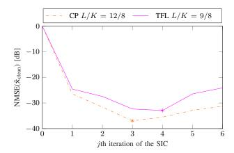
Fig. 6. NMSE of  $\hat{\mathbf{x}}_{\text{clean}}$  as a function of the number of iterations of the SIC for the radar scene described in Table I. Monte-Carlo simulation on 5,000 runs. QPSK symbols such that  $\sigma_{d-1}^2=1,\ K=64,\ M=32,\ \sigma^2=1,$  varying pulses and expansion factors L/K. Asterisks used to indicate minimum values.
