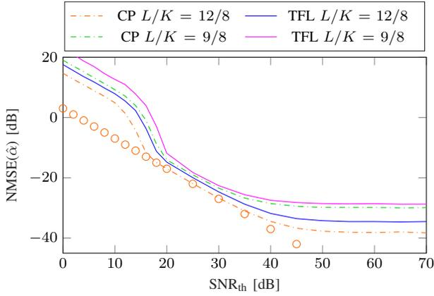
Fig. 3. NMSE of  $\hat{\alpha}$  obtained with our CLEAN-inspired procedure as a function of the theoretical SNR. Monte-Carlo simulation on 3,000 runs. QPSK symbols such that  $\sigma_{d-1}^2 = 1$ ,  $K = 64$ ,  $M = 32$ ,  $\sigma^2 = 1$ , varying  $L/K$  and pulses, target located in  $(l_0, f_d/L) = (35, 1/(4K))$  and  $\mathbb{E}\{\|\alpha\|^2\}$  defined by (8). Circle markers represent the NCRLB of  $\alpha$  in model (9) for CP-pulses with  $L/K = 12/8$ .
