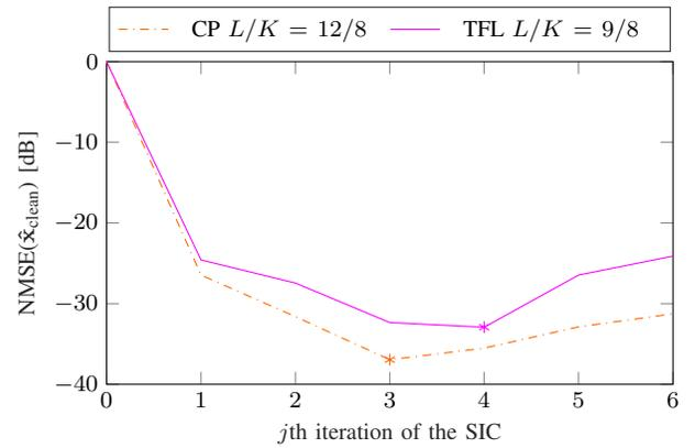
Fig. 6. NMSE of  $\hat{x}_{\text{clean}}$  as a function of the number of iterations of the SIC for the radar scene described in Table I. Monte-Carlo simulation on 5,000 runs. QPSK symbols such that  $\sigma_{d-1}^2 = 1$ ,  $K = 64$ ,  $M = 32$ ,  $\sigma^2 = 1$ , varying pulses and expansion factors  $L/K$ . Asterisks used to indicate minimum values.
