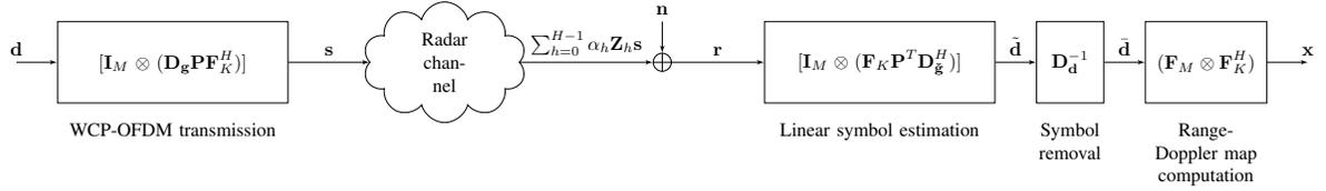
Fig. 2. Flowchart of the low-complexity WCP-OFDM radar transceiver.
