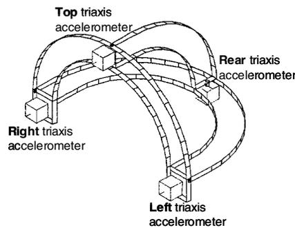
Figure 4 : Scheme of helmet equipped with 4 triaxis accelerometers
