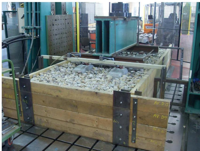
Figure 1 | Full-scale track model used in the present work.
