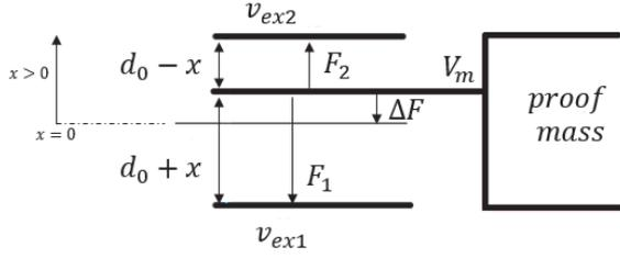
Fig. 1. Parallel plate model of a capacitive sensor.
