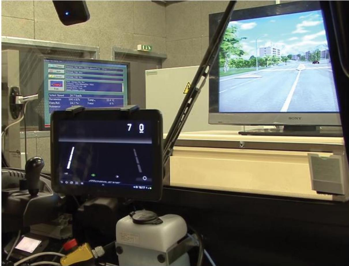
The last tested functionality is the V2V communication simulation. In this test, four virtual vehicles are simulated and their global positions are broadcasted by the 802.11p modem using CAM messages. Various DENM messages are also broadcasted by virtual vehicles. Another modem is embedded in the vehicle under test and receives these messages. An HMI is used to display this data to the driver, using a RADAR-like circular representation. A snapshot of the HMI is shown in [Figure 11.11](#).
