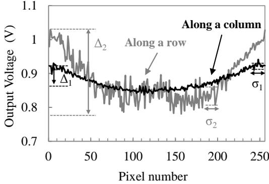
Fig. 3 Output Voltage along a column (black line) and a row (grey line) to show the  $V_{th}$   $SF_{PIXEL}$  non-uniformity due to the metal density difference effect. From these curves it was possible to extract the FPN non-uniformity,  $\Delta$ , and variability,  $\sigma$ .
