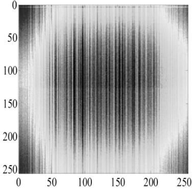
Fig. 2 ETF raw image (represented in logarithmic scale) captured at  $V_{DDRST}=2.8$  V (hard reset condition) after 1 MGy ( $\text{SiO}_2$ ) of irradiation in FURHI LOT1 #02 to show the arisen FPN with irradiation.
