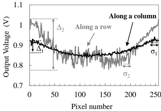
Fig. 3 Output Voltage along a column (black line) and a row (grey line) to show the  $V_{th}$   $SF_{PIXEL}$  non-uniformity due to the metal density difference effect. From these curves it was possible to extract the FPN non-uniformity,  $\Delta$ , and variability,  $\sigma$ .
