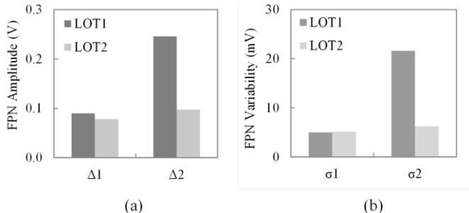
Fig. 7 Comparison of the FPN amplitudes (a) and variability (b) between FURHI LOT1 and FURHI LOT2 irradiated at 1 MGy(SiO<sub>2</sub>) and 1.1 MGy(SiO<sub>2</sub>) respectively.
