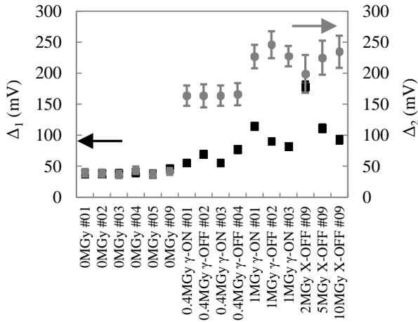
Fig. 4 Evolution of the average FPN amplitude along the columns ( $\Delta_1$ ) and along the rows ( $\Delta_2$ ) in the FURHI LOT1 circuits. The error bars of each point correspond to the variability, i.e.  $\sigma_1$  and  $\sigma_2$ .
