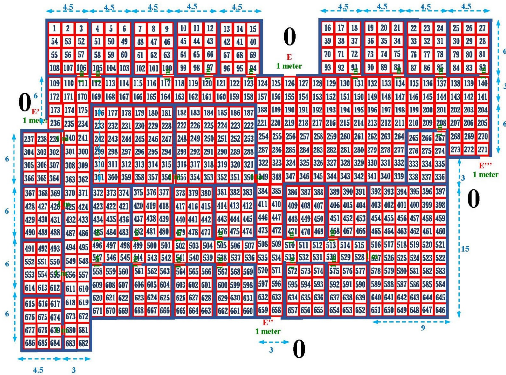
Figure 8. Plan embedding the Alan Turing building into square grids with a high resolution: 1.5 \times 1.5 cells.
