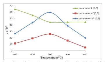
**Figure 7:** Evolution of the colorimetric parameters of Zn<sub>0.7</sub>Co<sub>0.3</sub>MoO<sub>4</sub> with the temperature.
