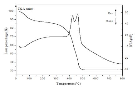
**Figure 2:** TGA–DTA curves of the Zn<sub>0.7</sub>Co<sub>0.3</sub>MoO<sub>4</sub> precursor
