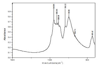
**Figure 4:** FT-IR spectra of Zn<sub>0.7</sub>Co<sub>0.3</sub>MoO<sub>4</sub> precursor powders treated at 500°C
