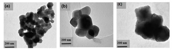
Figure 6: TEM Micrographs of  $Zn_{0.7}Co_{0.3}MoO_4$  treated at 500 ° C (a) / 700 ° C (b) and 800 ° C (c).
