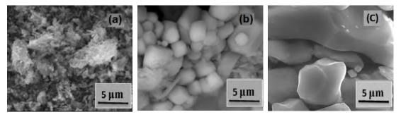
Figure 5: SEM micrograph of Zn<sub>0.7</sub>Co<sub>0.3</sub>MoO<sub>4</sub> treated at 500° C (a) / 700°C (b) and 800°C (c).
