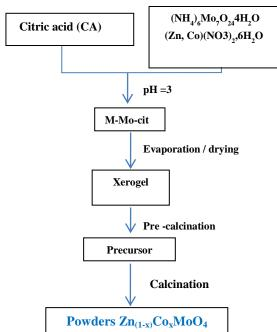
**Figure 1**: Flowchart of the synthesis of  $Zn_{1-x}Co_xMoO_4$   $0 \le x \le 0.3$  by the polymerizable complex method
