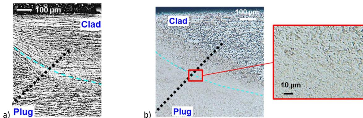
*Figure 3 – Weld micrographs: 14Cr (a) and 9Cr (b). The light blue dotted curve represents the approximate joint plane trace and the black dotted line represents the micro-hardness line-scans illustrated in Figure 5.*
