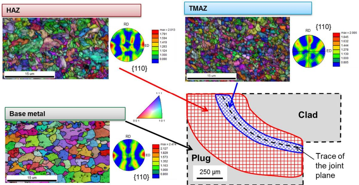
Figure 7 - IPF maps and  $\{110\}$  pole figures: illustration of the three different zones in terms of grain properties on a 9Cr weld schematic (before heat treatment); Base material (BM), Thermo-Mechanically Affected Zone (TMAZ) and Heat Affected Zone (HAZ).
