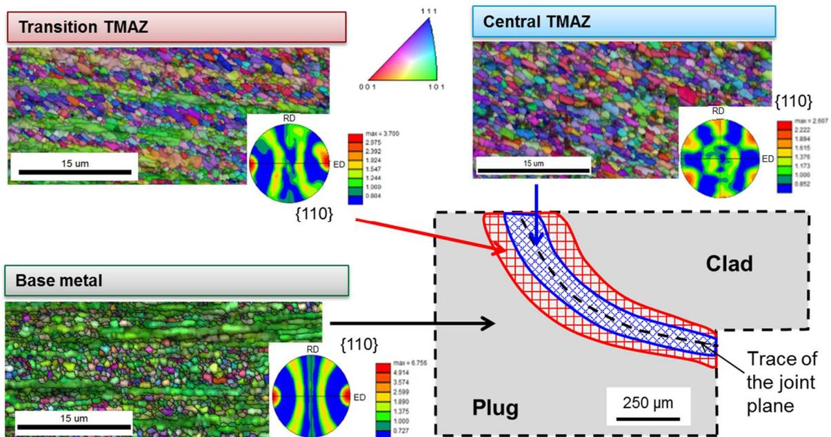
Figure 6 – IPF maps and  $\{110\}$  pole figures: illustration of the three different zones in terms of grain properties on a 14Cr weld schematic; Base material (BM), Transition Thermo-Mechanically Affected Zone (Transition TMAZ) and central Thermo-Mechanically Affected Zone (Central TMAZ).
