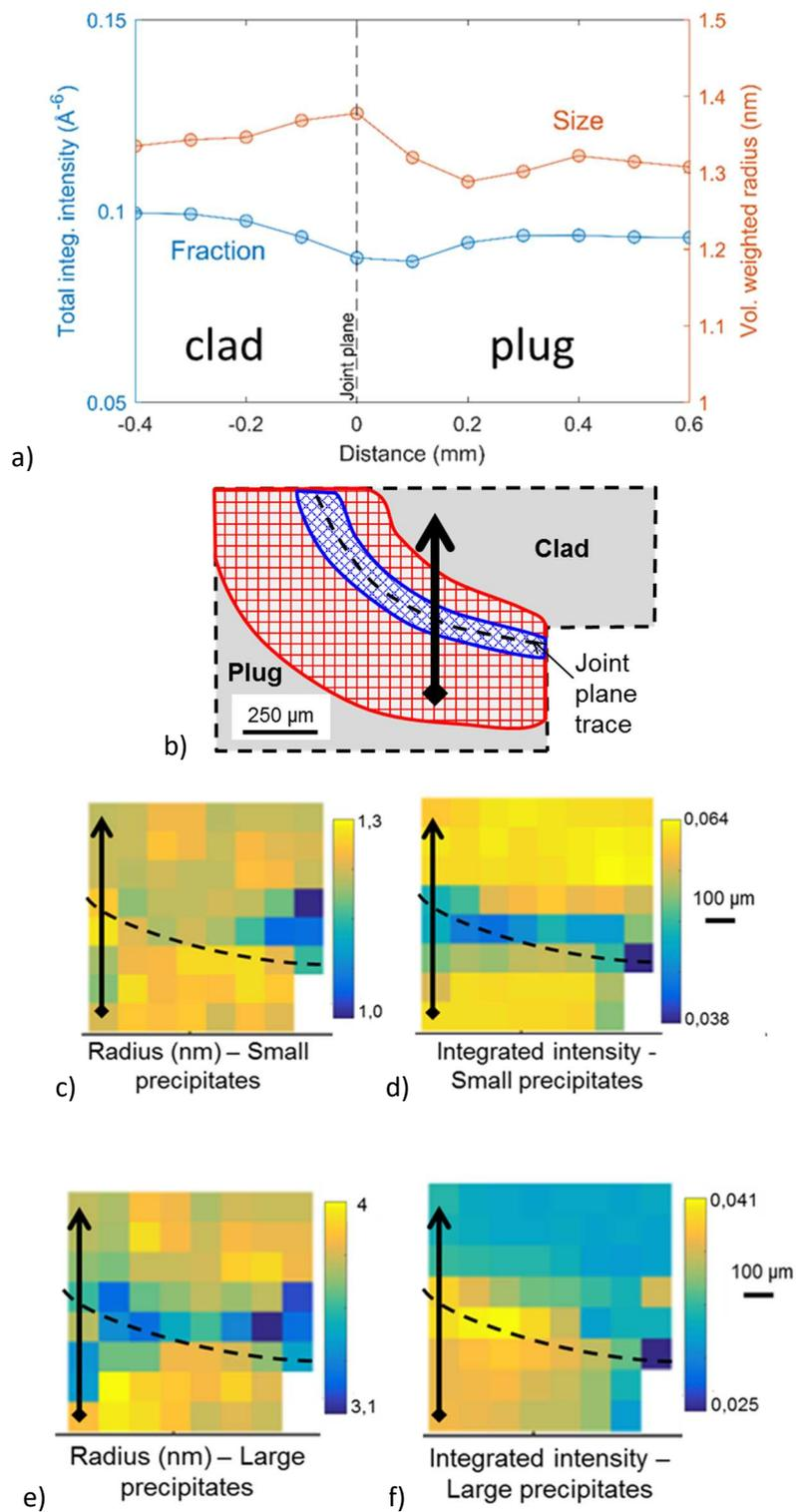
Figure 10 – 9Cr welded area: a) Precipitate radius (nm) and b) integrated intensity ( $\text{\AA}^{-6}$ ) evolution as a function of the distance to the joint plane along the dark arrow represented on the schema (c). SAXS cartographies for the small (d) and large (e) precipitate populations. More explanations can be found in sections 2.1 and 2.4.
