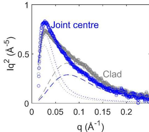
Figure 1 – Typical SAXS patterns of the clad zone as well as the joint center zone, represented as  $Iq^2$  vs  $q$  (Kratky plot) for the 9Cr weld. Circles are the experimental data and solid lines are the modeled intensity, which sums two contributions of smaller and larger precipitates (dashed and dotted lines).
