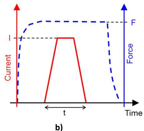
*Figure 2 – Central view of the resistance upset welding device part of CEA’s platform “ALTEA” (a), and representation of the welding parameters evolution with time (b).*
