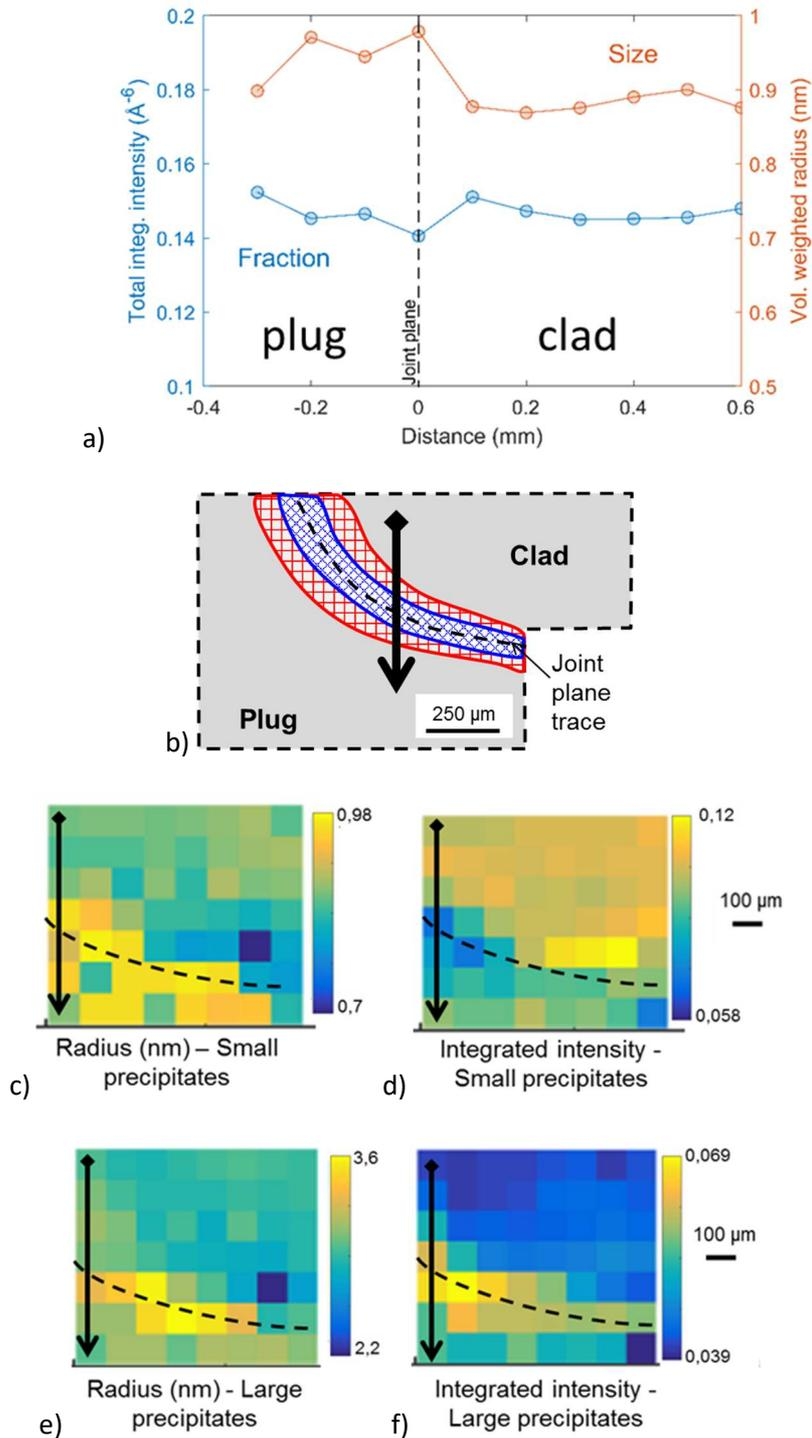
Figure 9 – 14Cr welded area: a) Precipitate radius (nm) and integrated intensity ( $\text{\AA}^{-6}$ ) evolution as a function of the distance to the joint plane along the dark arrow represented on the schema (b). SAXS maps for the small (c)-(d) and large (e)-(f) precipitate populations. More explanations can be found in sections 2.1 and 2.4.
