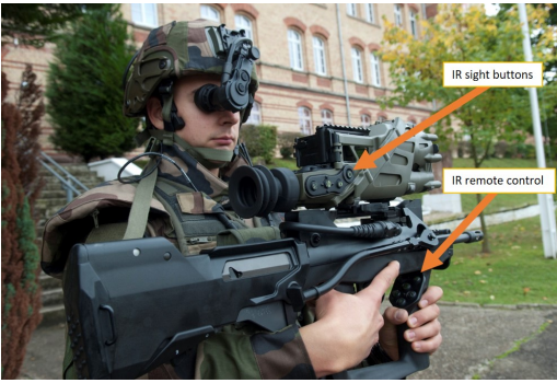
Figure 1: FELIN soldier equipped with the IR sight on the FAMAS rifle [3]
