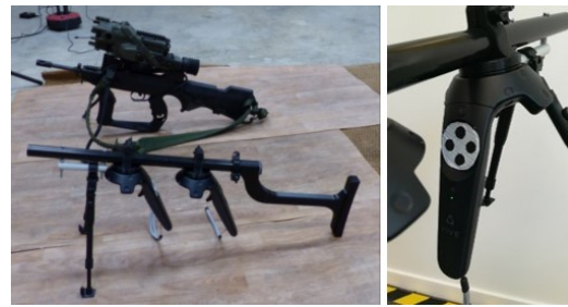
Figure 5: VR rifle support vs. FAMAS rifle (left) and adhesive mask added on the Vive controller (right)
