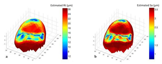
Fig. 2: Predicted roughness maps. (a) Rt 2D roughness predicted map. (b) Sa 3D roughness predicted map.
