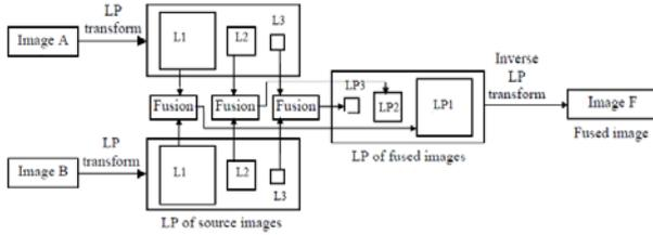
Figure 2. Scheme of LP fusion method.
