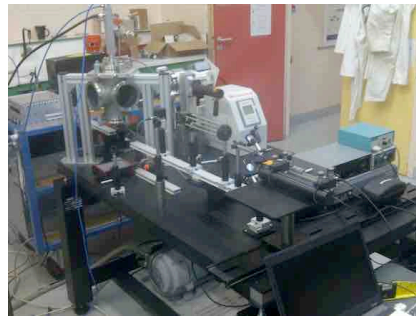
Figure 1. The cw visible laser assembly during installation and alignment.
