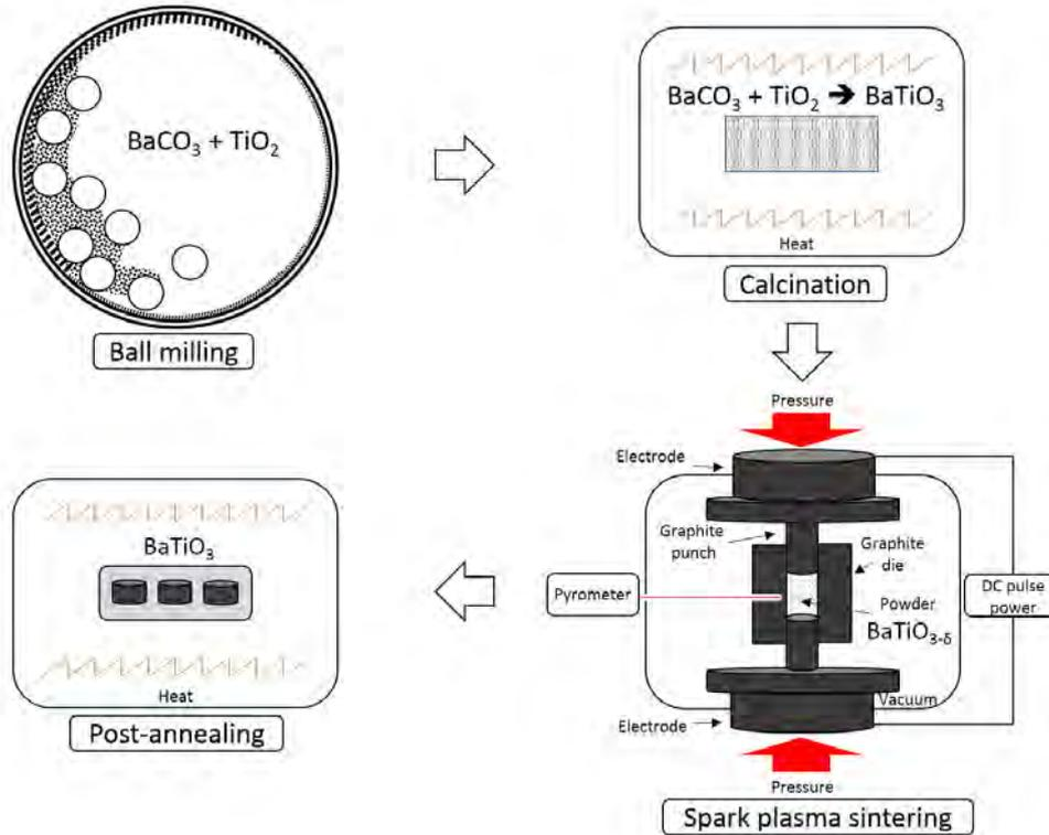
FIG 1: SCHEMA SHOWING THE CERAMICS ELABORATION PROCESS
