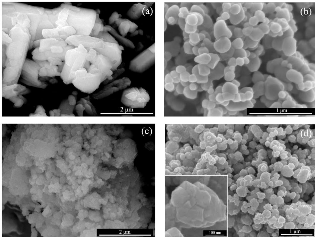
**FIG 6: SEM MICROGRAPHS OF: (A) COMMERCIAL BC AND (B)  $TiO_2$ , (C) AS MILLED MIXTURE BC AND  $TiO_2$  AND (D) BT POWDERS DERIVED FROM CALCINATION AT  $900^{\circ}C$  FOR 6H.**
