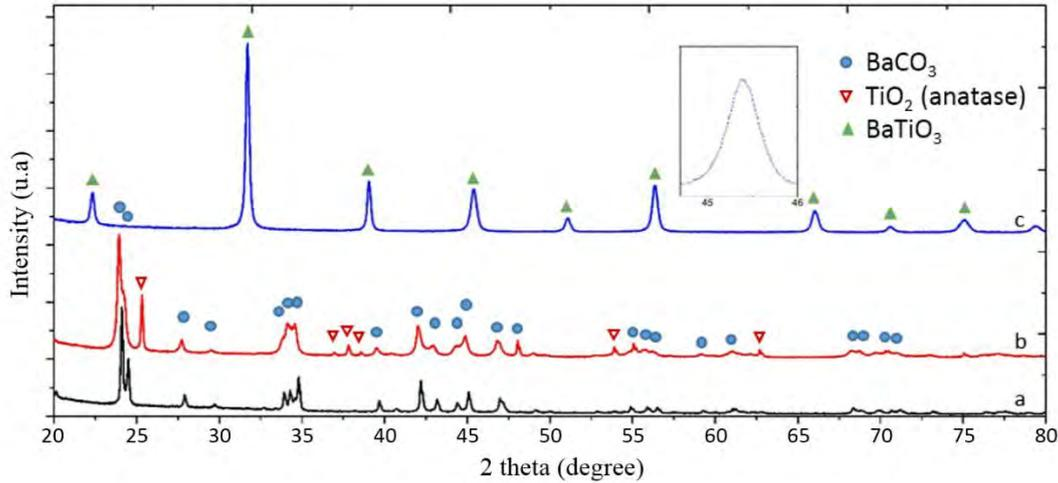
**FIG 4: XRD PATTERNS OF POWDERS: (A) COMMERCIAL BC AND THE 8H MILLED MIXTURE BC AND TiO<sub>2</sub> BEFORE (B) AND (C) AFTER CALCINATION (FOR 6H AT 900°C).**
