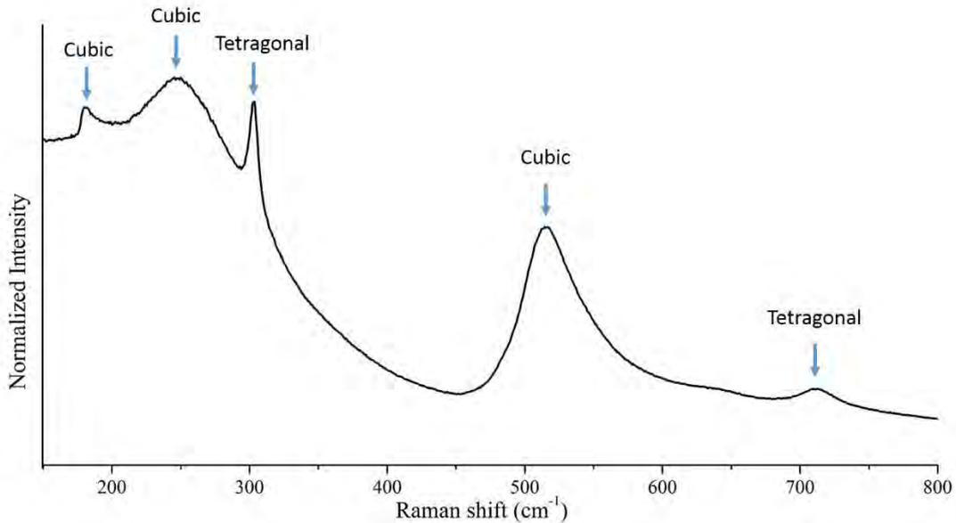
**FIG 5: RAMAN SPECTRUM OF BaTiO<sub>3</sub> POWDERS (OBTAINED BY 8H OF MILLING AT 350 RPM, AND CALCINATED FOR 6H AT 900<sup>0</sup> C).**
