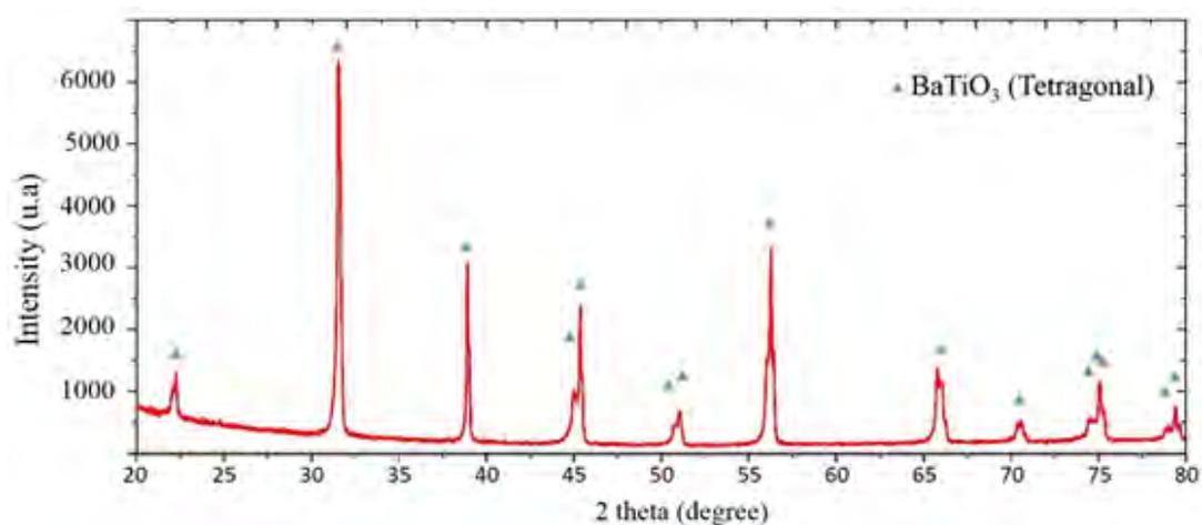
**FIG 7: XRD PATTERNS OF BT SINTERED BY SPS AT  $1112^{\circ}C$  (JCPDS No. 05-0626)**
