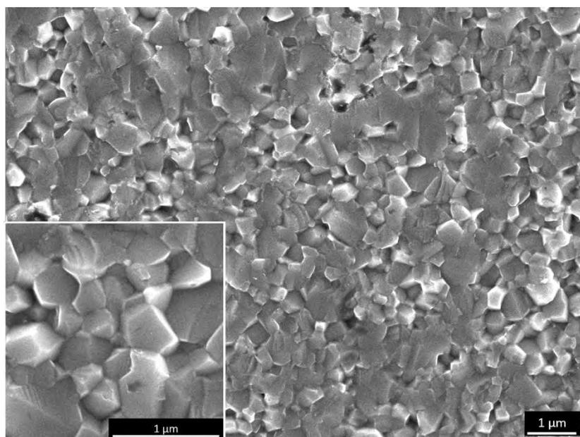
**FIG 8: SEM MICROGRAPHS OF A FRACTURE OF A BT CERAMIC**
