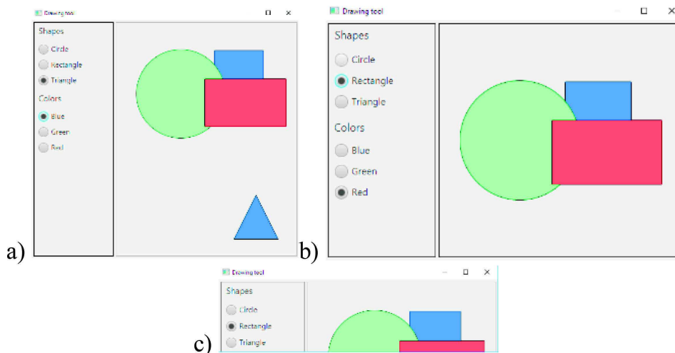
Fig. 5. The application window is (a) extended in height, (b) reduced in height after drawing the blue triangle and (c) reduced in height so radio buttons disappear (Color figure online)
