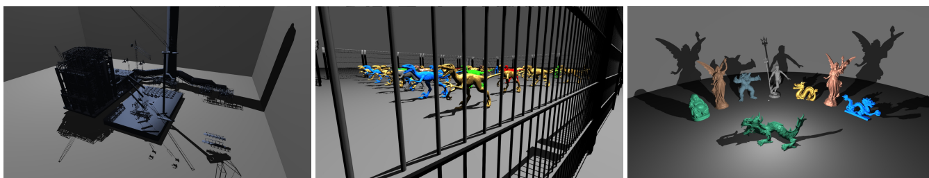
Figure 1: Three scenes rendered using our shadow algorithm. Left: Powerplant (12.7M triangles) 20ms. Middle : RaptorPark (30M triangles) 17ms. Right: ManyModels (73.8M triangles) 28ms.
