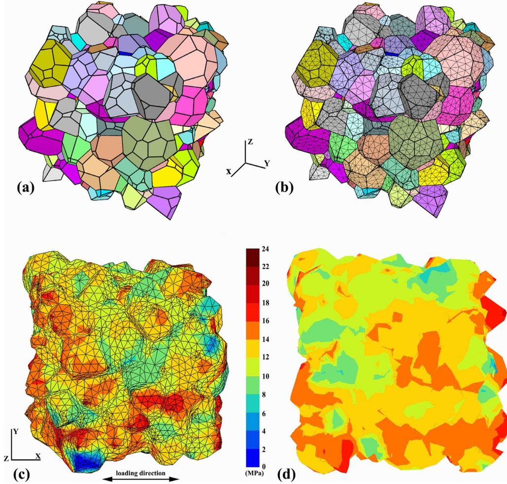
**Fig. 2.** (a) 3D periodic generation of a polycrystalline sample (343 grains); (b) periodic meshing with tetrahedral elements; (c) The von Mises stress distribution with strain of 0.1% after tensile test; (d) XY workplace of (c) on half Z.
