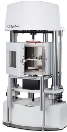
Fig.1 BOSE Electroforce 3230 DMTA equipped with a standard furnace [8]
