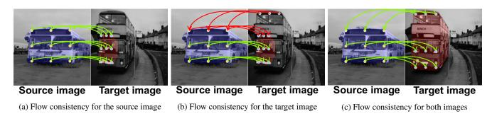
Figure 3: Symmetric loss. (a) Considering the flow consistency loss w.r.t a source image may cause a flow shrinkage problem. (b) We penalize inconsistent matches by computing the loss w.r.t a target image as well. (c) This symmetric loss allows to establish an object-to-object matching. We denote by green and red arrows consistent and inconsistent matches, respectively.
