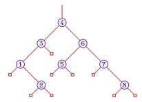
FIGURE 1. A binary tree of size 8 and the numbering of its nodes in the infix order.
