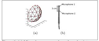
Figure 2. (a) Microphones array where the red points represent the probes position - (b) Two microphones spaced by 3 cm on the same probe
