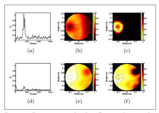
Figure 9. Error criterion for the off-centered source for SNR = 0 dB - Top: without FSM and without TRS: (a)  $E_n(t)$ , (b)  $T_1$  map, (c)  $T_2$  map; Bottom: with FSM and with TRS: (d)  $E_n(t)$ , (e)  $T_1$  map, (f)  $T_2$  map
