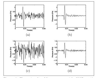
Figure 5. Time signals - Measurement with SNR=10 dB (a) and SNR=0 dB (c) - Comparison between the reference field (dashed line) and the reconstructed field with the FSM process (grey line) with SNR=10 dB (b) and SNR=0 dB (d)
