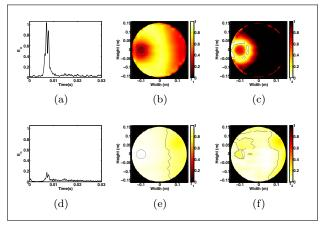
Figure 8. Error criterion for the off-centered source for SNR = 10 dB - Top: without FSM and without TRS: (a)  $E_n(t)$ , (b)  $T_1$  map, (c)  $T_2$  map; Bottom: with FSM and with TRS: (d)  $E_n(t)$ , (e)  $T_1$  map, (f)  $T_2$  map
