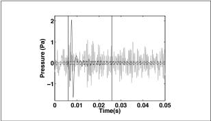
Figure 4. Measurement windowing for the SNR calculation
