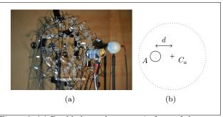
Figure 3. (a) Double-layered antenna in front of the moving baffled loudspeaker A (b) Loudspeaker A location in the source plane z = 0 and position of the antenna (dotted circle with a cross symbolizing the antenna center  $C_a$ )
