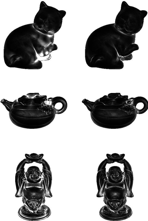
Fig. 9 Reprojection error, using white for 2.5 \cdot 10^{-3} and black for zero. Displayed are the results via (left) classic PS [41] and (right) the proposed method.
