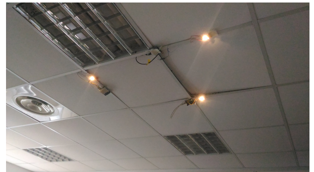
Figure 15: Experimental Tests in a real use case setup: Visible Light Communication Transmitters
