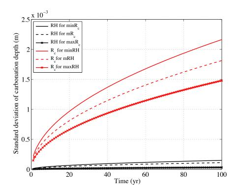
Figure 7. Standard deviation of output for several combinations of the constant and variable parameters, for the model of Oxand Petre-Lazar (2001).  $\min x_i = x_i$  is stated on its minimum value;  $\max x_i = x_i$  is stated on its maximum value;  $\max x_i = x_i$  is stated on its mean value;  $x_i = x_i$  varies on its range of values.
