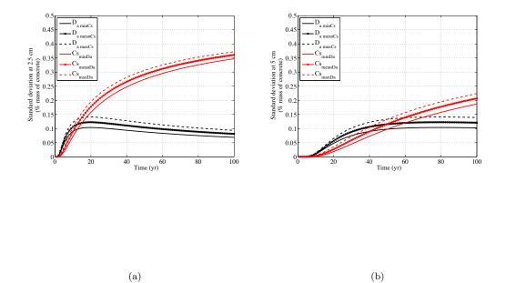
Figure 4. Evolution of output's standard deviation of the Collepardi model applied to the concrete C45, when the parameter  $C_s$  (respectively  $D_a$ ) varies and  $D_a$  (respectively  $C_s$ ) is stated at his minimum, mean and maximum value at 2.5 cm (a) and 5 cm (b)
