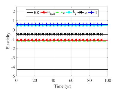
Figure 5. Elasticity of input parameters of the model of Hyvert for concrete C45
