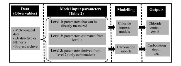
Figure 1. General representation of input parameters for analytical carbonation and chloride ingress models
