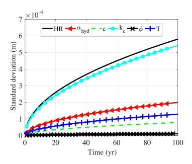
Figure 6. Standard deviation for the model of Hyvert for concrete C45
