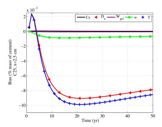
Figure 3. Bias of input parameters of the model of Leo for concrete C25 and at depth  $x=2.5~\mathrm{cm}$
