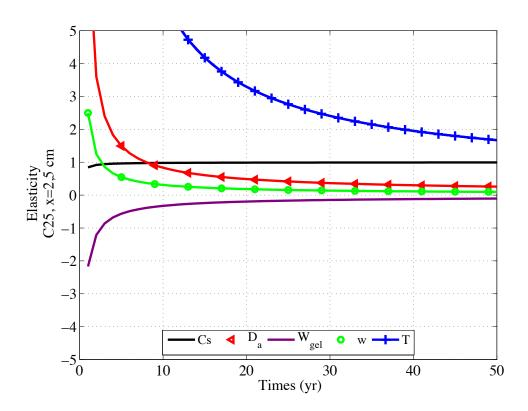
Figure 2. Elasticity of input parameters of the model of Leo for concrete C25 and at depth x=2.5 cm
