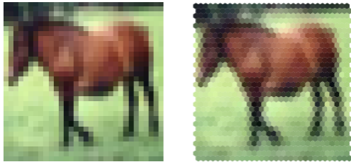
Figure 6: Example of an image from CIFAR-10 dataset resampled to hexagonal grid.
