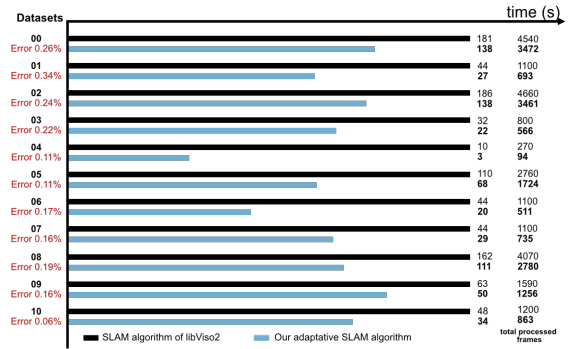
Figure 9: Evaluation of adaptive SLAM algorithm compared to libviso2 on the KITTI dataset. This array clearly highlights the saved computational time on real data. It also confirms that the error is negligible in comparison.
