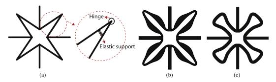
**Fig. 1.** (a) Star-shaped auxetics and the mechanism at the vertices. The study in Ref. [1] focuses on (b) the design of exterior petal boundary subjected to a geometric width constraint, while the study in this work focus on (c) the optimal shape form and part width of tetra-petals auxetics.
