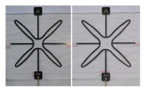
Fig. 17. A unit sample (case A9) before (left) and after (right) tension loading. The in-plane bar/petal width is 5.1 mm, much larger than the out-of-plane thickness of 1.6 mm, which is a key factor of the out-of-plane buckling under tension.
