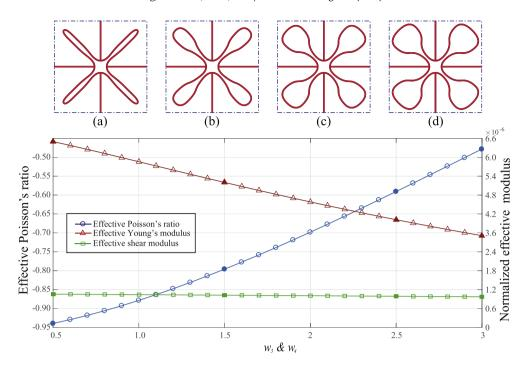
**Fig. 4.** Parameter analysis with respect to  $w_3$  and  $w_4$  that control the curvature of the petal tips. The solid symbols denote the effective properties for structures (a)–(d), corresponding to  $w_3 = w_4 = 0.5, 1.5, 2.5, \text{and } 3.0, \text{ respectively.}$
