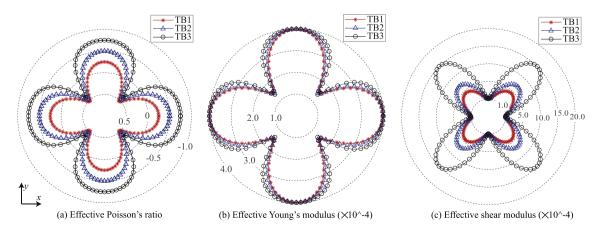
Fig. 14. Effective (a) Poisson's ratios, (b) Young's moduli and (c) shear moduli along different directions for design cases TB1, TB2 and TB3.
