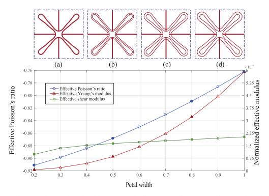
**Fig. 5.** Parameter analysis with respect to the petal width  $d_2$ . The solid symbols denote the effective properties for structures (a)–(d), corresponding to  $d_2 = 0.2, 0.5, 0.8$ , and 1.0, respectively.
