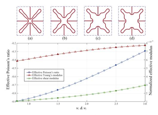
**Fig. 3.** Parameter analysis with respect to  $w_1$  and  $w_2$  that control the opening and re-entrant ratio of the petals. The solid symbols denote the effective properties for structures (a)–(d), corresponding to  $w_1 = w_2 = 0.8, 1.5, 2.5, \text{and } 3.0$ , respectively.
