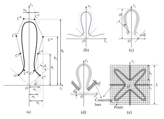
**Fig. 2.** Parameterization scheme for the tetra-petal-shaped auxetics: (a) interior petal boundary parameters, (b) exterior petal boundary generated by NURBS offsetting, (c) NURBS patch of a parent petal, and (d) connecting bars placement. The design in (e) corresponds to parameters of  $w_1 = 1.5$ ,  $w_2 = 1.0$ ,  $w_3 = 1.0$ ,  $w_4 = 0.5$ ,  $h_4 = 10.25$ ,  $h_4 = 10.2$
