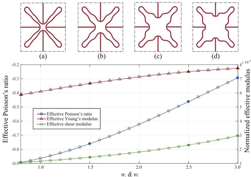
Fig. 3. Parameter analysis with respect to  $w_1$  and  $w_2$  that control the opening and re-entrant ratio of the petals. The solid symbols denote the effective properties for structures (a)–(d), corresponding to  $w_1 = w_2 = 0.8, 1.5, 2.5$ , and  $3.0$ , respectively.
