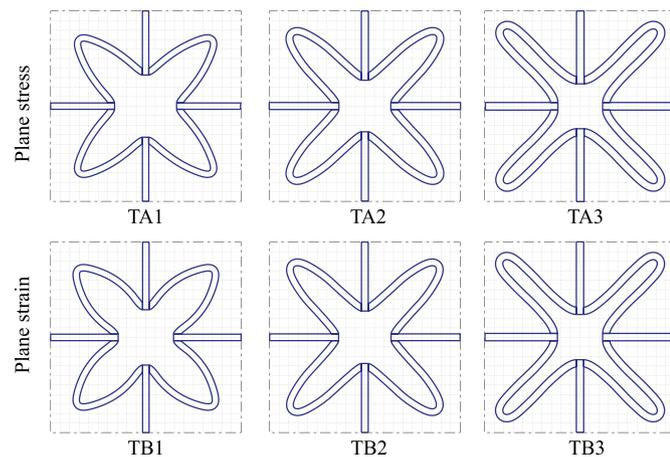
**Fig. 10.** Tunable material property designs with different target Poisson's ratios of  $-0.75$  (TA1 and TB1),  $-0.50$  (TA2 and TB2) and  $-0.25$  (TA3 and TB3), respectively, with TA1–3 for plane stress cases and TB1–3 for plane strain cases. The depicted designs match the target Poisson's ratios exactly with the same normalized Young's modulus of  $\bar{E}^Y = 4.0 \times 10^{-4} E_0^Y$  and shear modulus of  $\bar{G} = 1.0 \times 10^{-4} E_0^Y$ .
