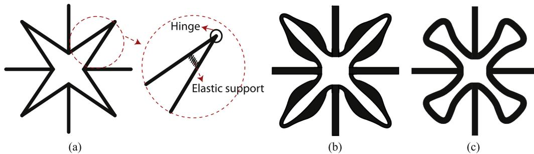
**Fig. 1.** (a) Star-shaped auxetics and the mechanism at the vertices. The study in Ref. [1] focuses on (b) the design of exterior petal boundary subjected to a geometric width constraint, while the study in this work focus on (c) the optimal shape form and part width of tetra-petals auxetics.
