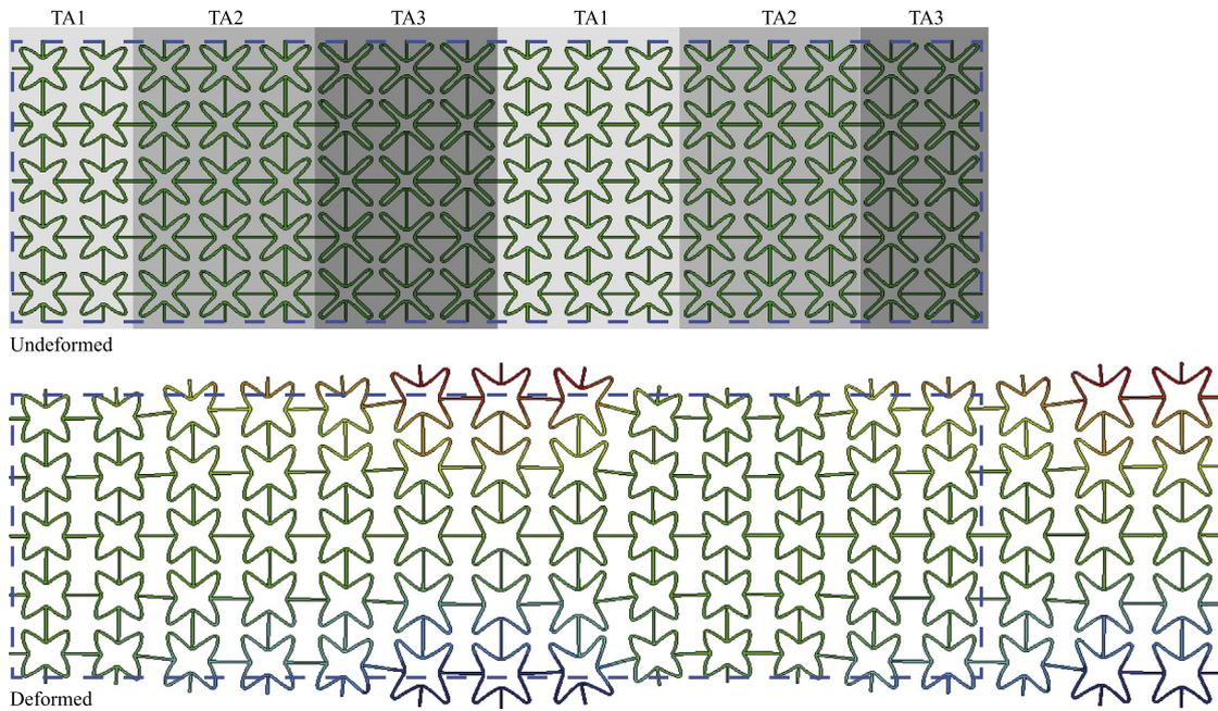
**Fig. 11.** A functionally graded structure built from unit structures of TA1, TA2 and TA3. The blue dash rectangular describes the region of the undeformed structure. The deformation is scaled by a factor of 5. The structure exhibits a variable vertical expansion at different locations under tensile deformation, which can be utilized for the design of shape matching structures, e.g., in Ref. [47].
