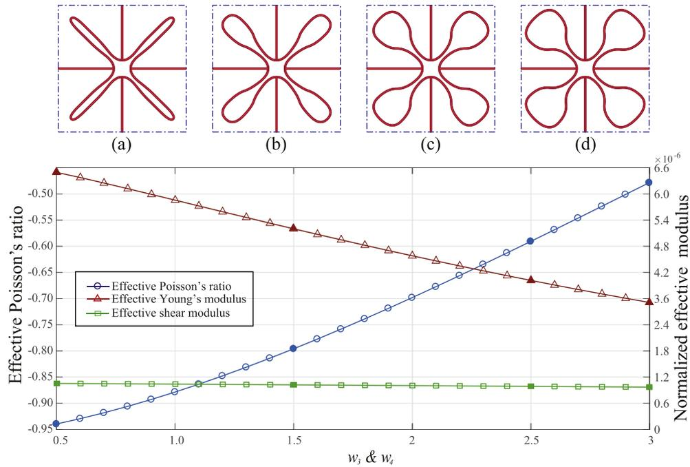
**Fig. 4.** Parameter analysis with respect to  $w_3$  and  $w_4$  that control the curvature of the petal tips. The solid symbols denote the effective properties for structures (a)–(d), corresponding to  $w_3 = w_4 = 0.5, 1.5, 2.5,$  and  $3.0$ , respectively.
