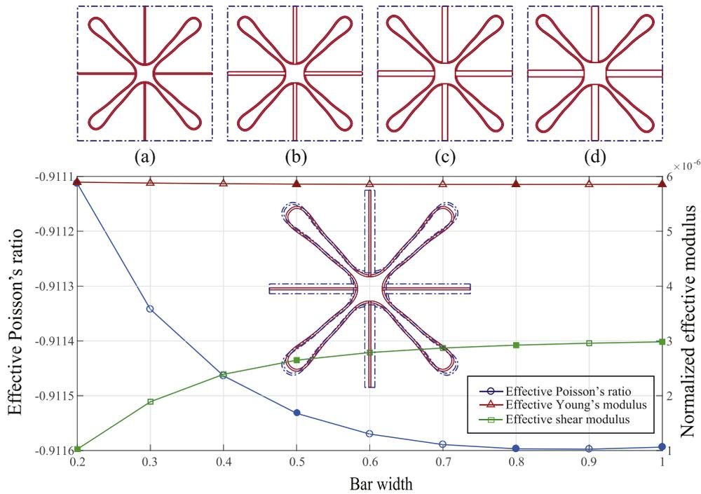
**Fig. 6.** Parameter analysis with respect to the width of the connecting bars  $d_3$ . The change of the effective NPR and the normalized effective Young's modulus is relatively small. The solid symbols denote the effective properties for structures (a)–(d), corresponding to  $d_3 = 0.2, 0.5, 0.8,$  and  $1.0$ , respectively. The overlay of (a) and (d) shown in the graph depicts a slight change in petal tip positioning.
