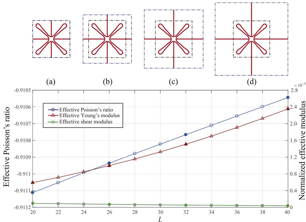
**Fig. 7.** Parameter analysis with respect to the unit side length  $L$  that is inversely proportional to the petal size ratio ( $H/L$ ). The decrement of the effective NPR is relatively small. The solid symbols denote the effective properties for structures (a)–(d), corresponding to  $L = 20, 26, 32,$  and  $40$ , respectively.
