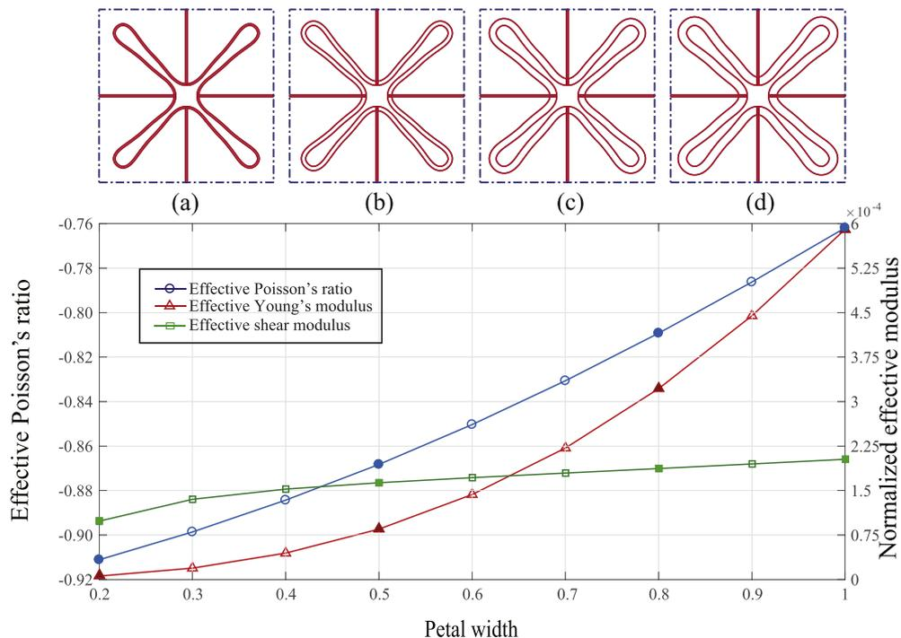
**Fig. 5.** Parameter analysis with respect to the petal width  $d_2$ . The solid symbols denote the effective properties for structures (a)–(d), corresponding to  $d_2 = 0.2, 0.5, 0.8,$  and  $1.0$ , respectively.
