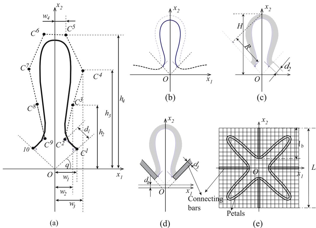
**Fig. 2.** Parameterization scheme for the tetra-petal-shaped auxetics: (a) interior petal boundary parameters, (b) exterior petal boundary generated by NURBS offsetting, (c) NURBS patch of a parent petal, and (d) connecting bars placement. The design in (e) corresponds to parameters of  $w_1 = 1.5$ ,  $w_2 = 1.0$ ,  $w_3 = 1.0$ ,  $w_4 = 0.5$ ,  $h_4 = 10.25$ ,  $d_1 = 0.5$ ,  $d_2 = 0.5$ , and  $d_3 = 0.5$ .
