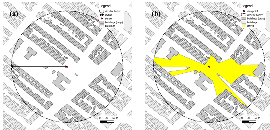
Fig. 2: Two different methods of delineating surrounding spaces: (a) Circular buffer. (b) Isovist.
