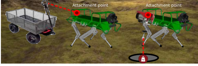
Fig. 16. Use cases for load estimation: (left) the robot is pulling a cart, (right) the robot is pulling up a payload.
