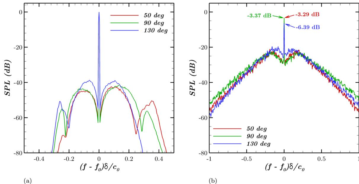
Figure 9: Comparison of the SPL at different microphone positions for the cases (a)  $f_0 = c_0/\delta$  and (b)  $f_0 = 8c_0/\delta$ .
