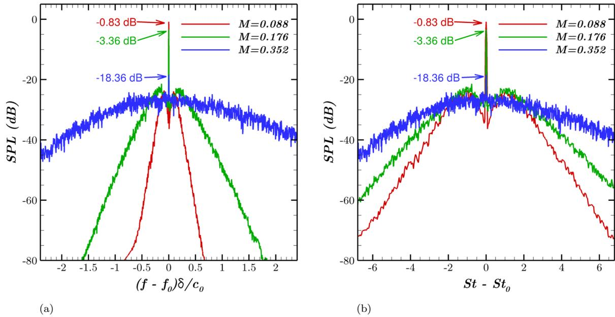
Figure 11: Comparison of the SPL at different convection Mach numbers for a source frequency  $f_0 = 8c_0/\delta$  (a) plotted versus the frequency and (b) plotted versus the Strouhal number  $St = f\delta/U_0$ .
