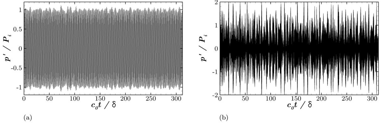
Figure 6: Pressure fluctuation signals over the duration of a segment of the periodogram at the microphone position  $\theta = 90^\circ$  for the source frequencies (a)  $f_0 = c_0/\delta$  and (b)  $f_0 = 8c_0/\delta$ .
