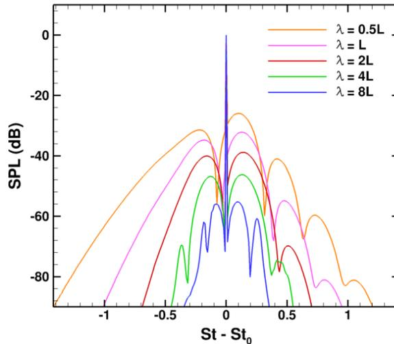
Figure 8: SPL obtained for the scattering by a single inviscid vortex of core size  $L$  convected by a uniform mean flow at  $M = 0.176$  for different source frequencies (or wavelength in the legends). Results from Clair and Gabard.<sup>10</sup>
