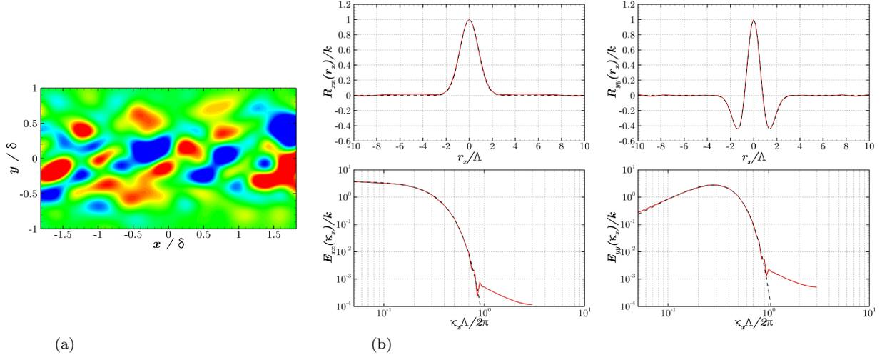
Figure 2: Example of a turbulent field synthesized using the *RPM*. (a) Snapshot of the  $u_t/c_0$  velocity fluctuation (levels between  $\pm 0.025$ ). (b) Correlations and one-dimensional spectra: (—) *RPM* and (---) analytical solutions.
