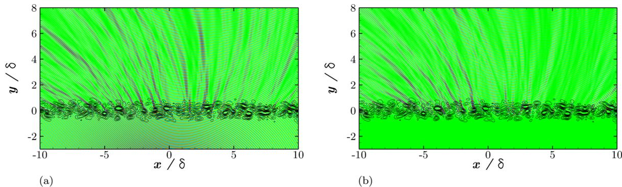
Figure 5: Snapshots of (a) the total pressure fluctuation  $p'/P_i$  (levels between  $\pm 2$ ) and (b) the scattered pressure fluctuation  $p'_s/P_i$  (levels between  $\pm 2$ ) for the source frequency  $f_0 = 8c_0/\delta$ . The lines are the  $u_t/c_0$  turbulent velocity component (levels between  $\pm 0.05$ ).
