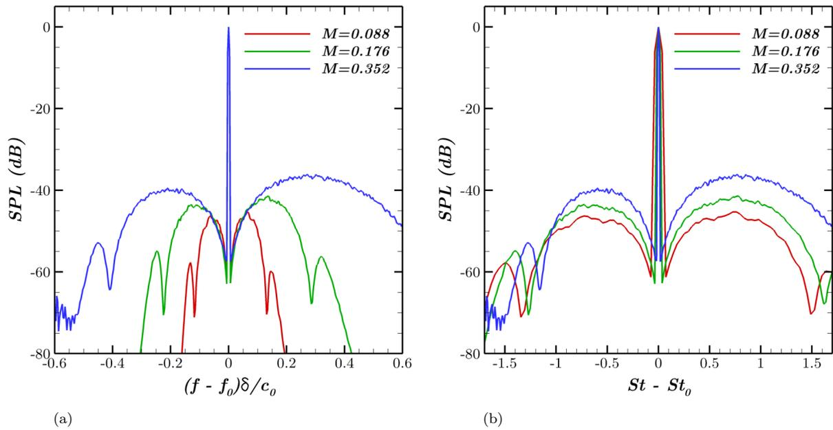
Figure 10: Comparison of the SPL at different convection Mach numbers for a source frequency  $f_0 = c_0/\delta$  (a) plotted versus the frequency and (b) plotted versus the Strouhal number  $St = f\delta/U_0$ .
