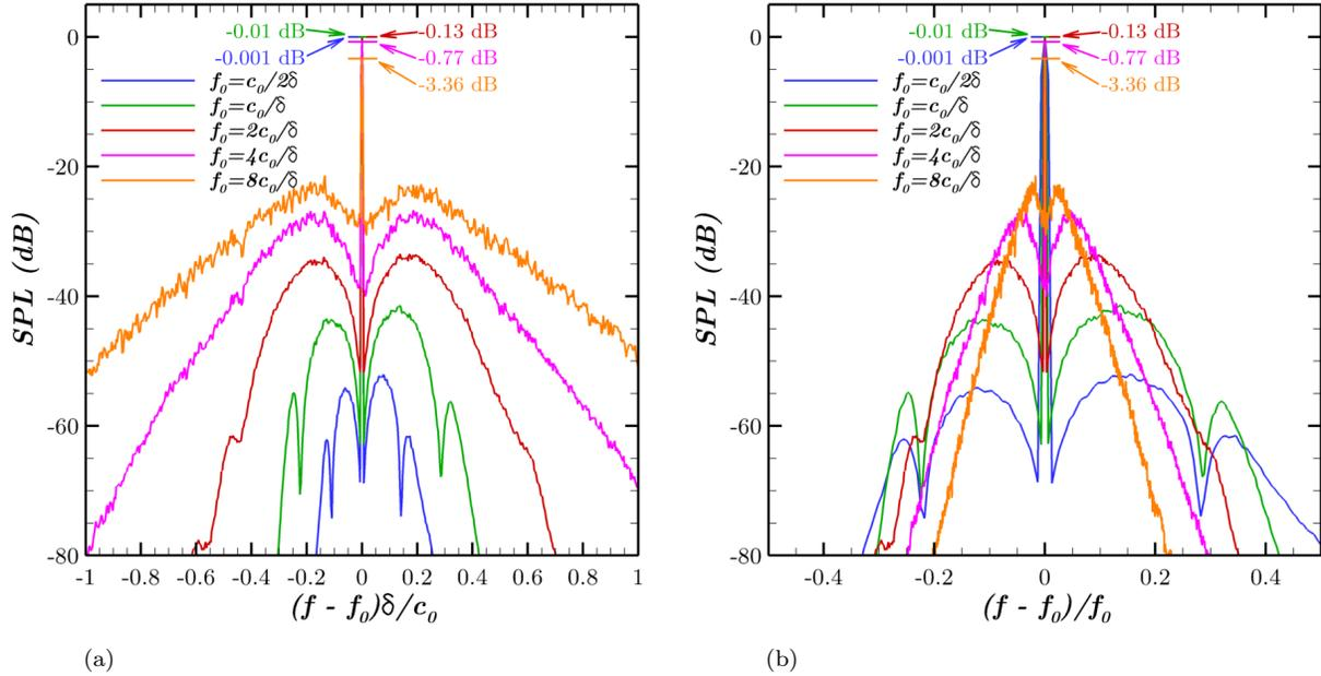
Figure 7: Comparison of the SPL at the microphone position  $\theta = 90^\circ$  for different source frequencies (a) plotted versus the frequency and (b) plotted versus the frequency reduced by the source frequency  $f_0$ .
