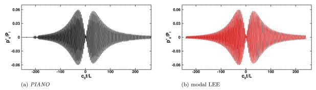
Figure 12: Time signals of the scattered pressure recorded for the scattering of a plane wave by a convected vortex.
