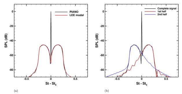
Figure 13: SPL of the scattered pressure recorded by the microphone for the scattering of a plane wave by a convected vortex. (a) Comparison between *PIANO* and the modal LEE method. (b) SPL of the time signal splitted at t = 0.
