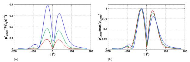
Figure 8: RMS scattered pressure obtained with different values of  $M_v$  at  $r = 2.5\lambda_0$  around the vortex (a) without normalization and (b) normalized by their maximum values. (-----)  $M_v = 0.0625$ , (------)  $M_v = 0.125$  and (----------)  $M_v = 0.25$ .
