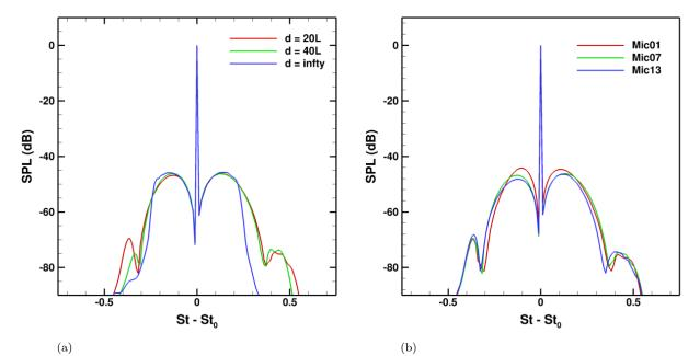
Figure 15: Effects of the distance between the source and the vortex path. (a) SPL at the central microphone location for the different source distances (b) SPL at different microphone locations for the reference case (d = 20L).
