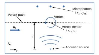
Figure 1: Schematic of the scattering of an acoustic radiation by a convected vortex.
