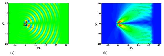
Figure 4: *PIANO* results: (a) Snapshot of the scattered pressure fluctuation field  $p'_s/P_i$  (levels between  $\pm 0.25$ ). The lines represent the vortex axial velocity (contours between  $\pm 0.125$ , negative values in dashed lines). (b) RMS field of the scattered pressure  $p'_{RMS}/P_i$  (levels between 0 and 0.2).
