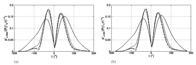
Figure 6: Comparison between the RMS scattered pressure obtained (a) with *PIANO* and (b) with the modal LEE method at different radii: (---)  $r = 0.5\lambda_0$ , (---)  $r = \lambda_0$ , (---)  $r = 1.5\lambda_0$ , (---)  $r = 2\lambda_0$ , (---)  $r = 2.5\lambda_0$ .
