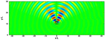
Figure 11: Snapshot of pressure scattered by a convected vortex for an incident plane wave propagating in the +y-direction. Color levels:  $p'_s/P_i$  between  $\pm 0.075$  and lines: vortex axial velocity between  $\pm 0.05$ .
