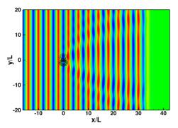
Figure 3: Snapshot of the total pressure fluctuation field  $p'/P_i$  (levels between  $\pm 1$ ). The lines represent the vortex axial velocity (contours between  $\pm 0.125$ , negative values in dashed lines).
