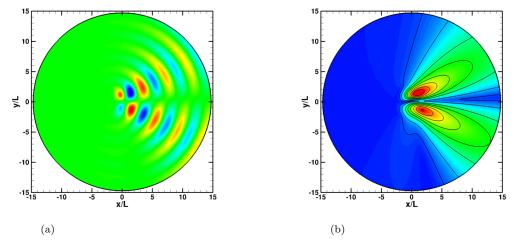
Figure 5: modal LEE results: (a) Snapshot of the scattered pressure fluctuation field  $p'_s/P_i$  (levels between  $\pm 0.25$ ) and (b) RMS field of the scattered pressure  $p'_{RMS}/P_i$  (levels between 0 and 0.2).
