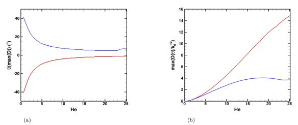
Figure 10: Evolution of (a) the angular positions and (b) the magnitudes of the maxima of the scattered directivity with the incident wave Helmholtz number for (----)  $\theta > 0^{\circ}$  and (-----)  $\theta < 0^{\circ}$ .
