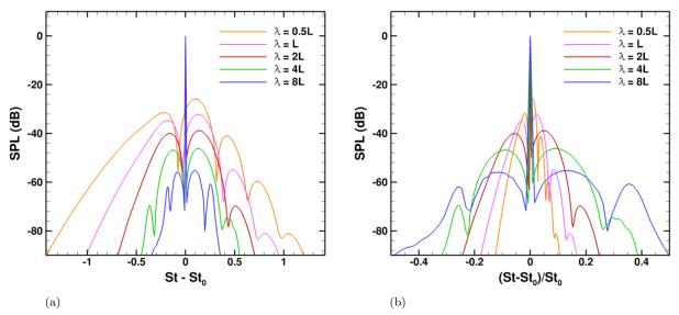
Figure 19: SPL of the scattered field at the central microphone location for the different values of  $\lambda_0$ , (a) as a function of the Strouhal number and (b) as a function of the reduced Strouhal number.
