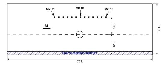
Figure 14: Schematic of the computational domain considered for the parametric study with PIANO.
