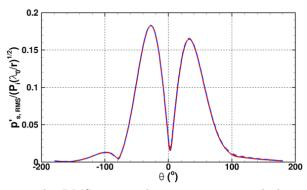
Figure 7: Comparison between the RMS scattered pressure on a circle located at  $r = 2.5\lambda_0$  around the vortex, (-----) without enforcing the vortex pressure and density fields ( $\rho_t = p_t = 0$ ) and (---) with the pressure and density fields decribed in Eq. (1).
