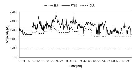
Fig. 1. Evolution of Static Line Rating and Real Line Rating over a 3-day period
