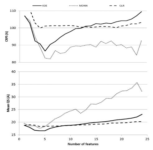
Fig. 3. Comparison of the CRPS and the QS obtained with the MDNN and the KDE, with a variable number of features selected through PCA
