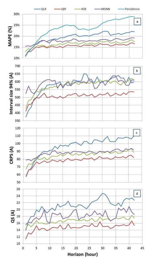
Fig. 6. Comparison of the evaluation criteria for the four considered models, depending on the forecast horizon.
