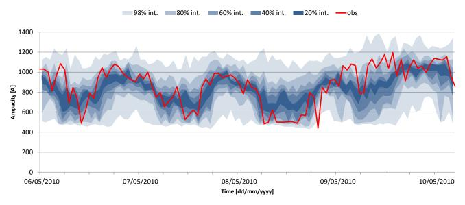
Fig. 2. Example of the RTLR probabilistic forecast over a four days period with the QRF model.
