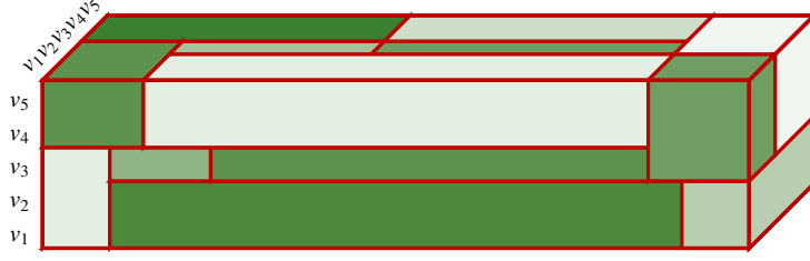
Figure 5: Multistream compression, that is the Cartesian partitioning of V \times V \times T , consists in the natural tridimensional generalisation of multigraph compression, that is the Cartesian partitioning of V \times V .
