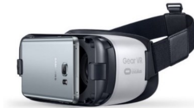
Figure 2. The SamsungGear (Samsung, Seoul, South Korea) consists in a plastic mask in which we insert a smartphone.
