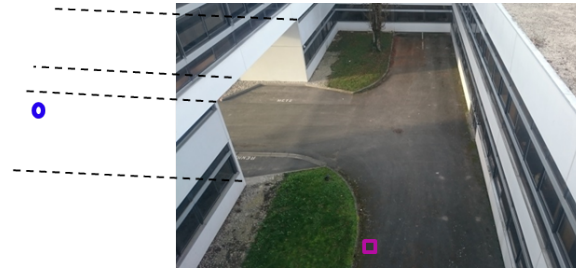
Fig. 11: Photo of the T-junction for the measurement campaign. The radar was placed at the end of the tunnel (blue circle). The target walked toward the right tail of the T (pink rectangle).
