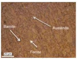
Figure 1: Microstructure of the TRIP 780 steel. Austenite corresponds to white grains.
