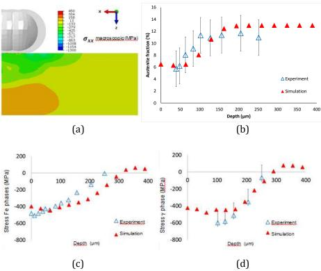
Figure 5: Shot peening of the non-deformed TRIP 780 steel. Simulated macroscopic stress in x direction (a). Experimental vs. simulated austenite volume fraction profile (b), residual stress profiles in the BCC phases (c) and in austenite  $\gamma$  (d).
