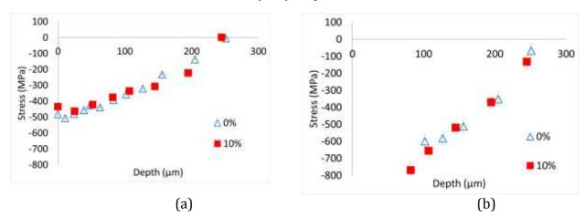
Figure 3: Residual stress profile in the BCC phases as a function of depth for as-received (0%) and prestrained (10%) samples after SP
