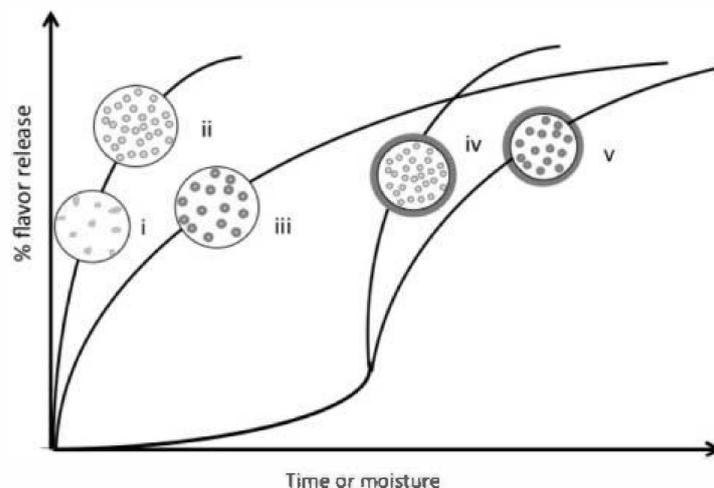
**Figure 4.** Scheme of release profile depending on the morphology of the delivery system obtained by extrusion.
