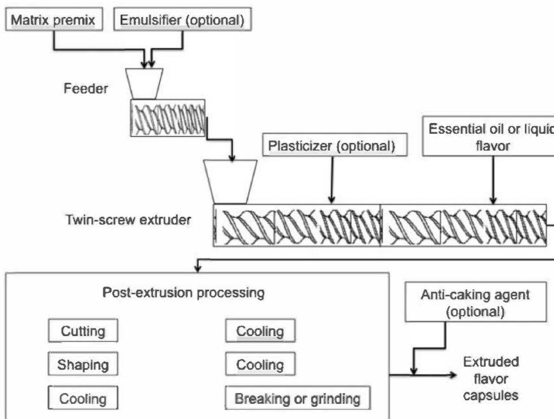
**Figure 6.** Scheme of flavor encapsulation by melt extrusion using a Twin-screw extruder (adapted from Ubbink and Schoonman<sup>16</sup>).
