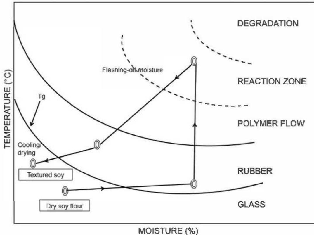
**Figure 7.** State diagram showing transformations of proteins during the wetting, heating, cooling, and drying stages of extrusion cooking (adapted from Kokini et al.<sup>111</sup>).
