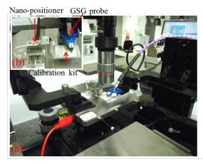
Fig. 1. (a) Modified Wafer probe station for on-wafer measurements in the range 0.05-50 GHz. (b) Mounting of the sample holder on the nano-positioning stage.
