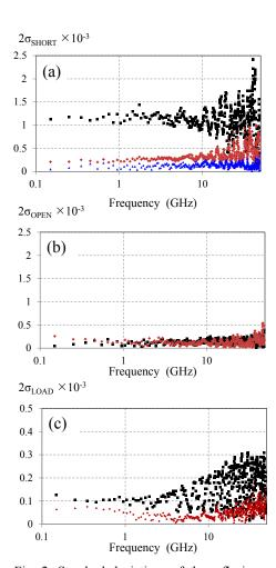
Fig. 2. Standard deviations of the reflecion coefficient  $S_{11}$  as a function of the frequency (loads are respectively short, open and load ISS standards) determined for n consecutive measurements (piezo-electric positioning:  $\bullet$  n=15 and  $\blacktriangle$  n=4, mechanical positioning:  $\blacksquare$  n=15).
