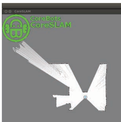
Figure 8. Observed environment by the robot though Core SLAM units
