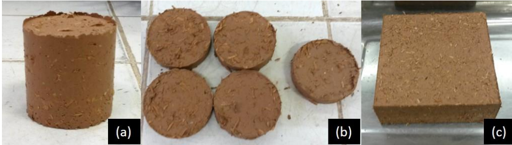
Figure 3. (a) Cylindrical specimens, (b) microbial proliferation specimens and (c) rectangular prismatic specimens
