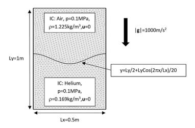
Figure 19: 2D single-mode Rayleigh-Taylor instability computational set up.
