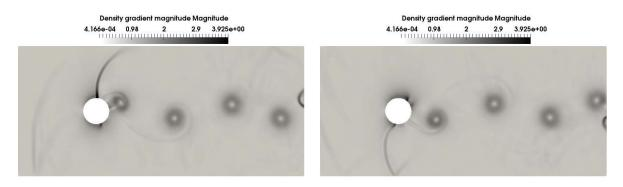
Figure 8: Single-phase transonic flow past a circular cylinder. Contours of density gradients magnitude when periodic regime is reached.
