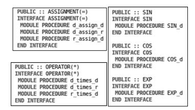
Figure 3: Example of operator and function overloading. Interface blocks allowing the use of the symbols =,\* and the intrinsic functions SIN,COS and EXP whether the arguments are of type REAL or AutoDiffType or a mix of both.
