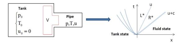
Figure 21: Tank-inlet boundary condition description.
