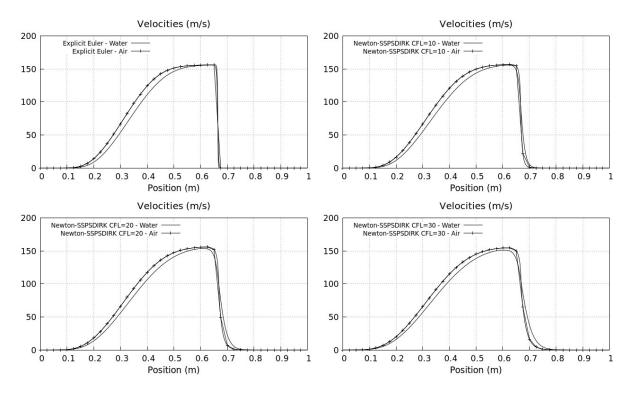
Figure 14: Water-air mixture shock tube with pressure relaxation and drag effects. Water and air velocities using explicit and implicit time integrators.
