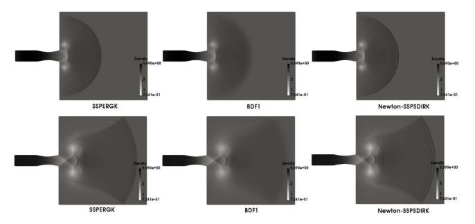
Figure 18: 2D jet at time t=14ms (top) and t=21ms (bottom). Mixture density contours.
