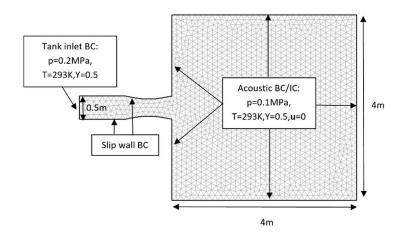
Figure 17: 2D sonic jet computational set-up.
