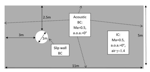
Figure 7: Single-phase transonic flow past a circular cylinder. Computational set-up.
