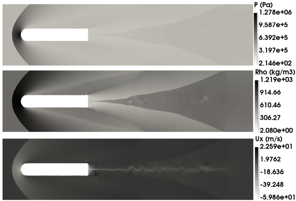
Figure 4.7- Computations of the moving body in two-phase mixture with the coupling method. Density, velocity and pressure contours are shown at time 0.5 s and computed with a mesh involving 302 812 cells corresponding to an average space step of 3 cm and CFL=0.8. The rigid body is tracked with the Level-Set function and Overbee limiter while the other flow variables are computed with the Minmod limiter and MUSCL scheme.
