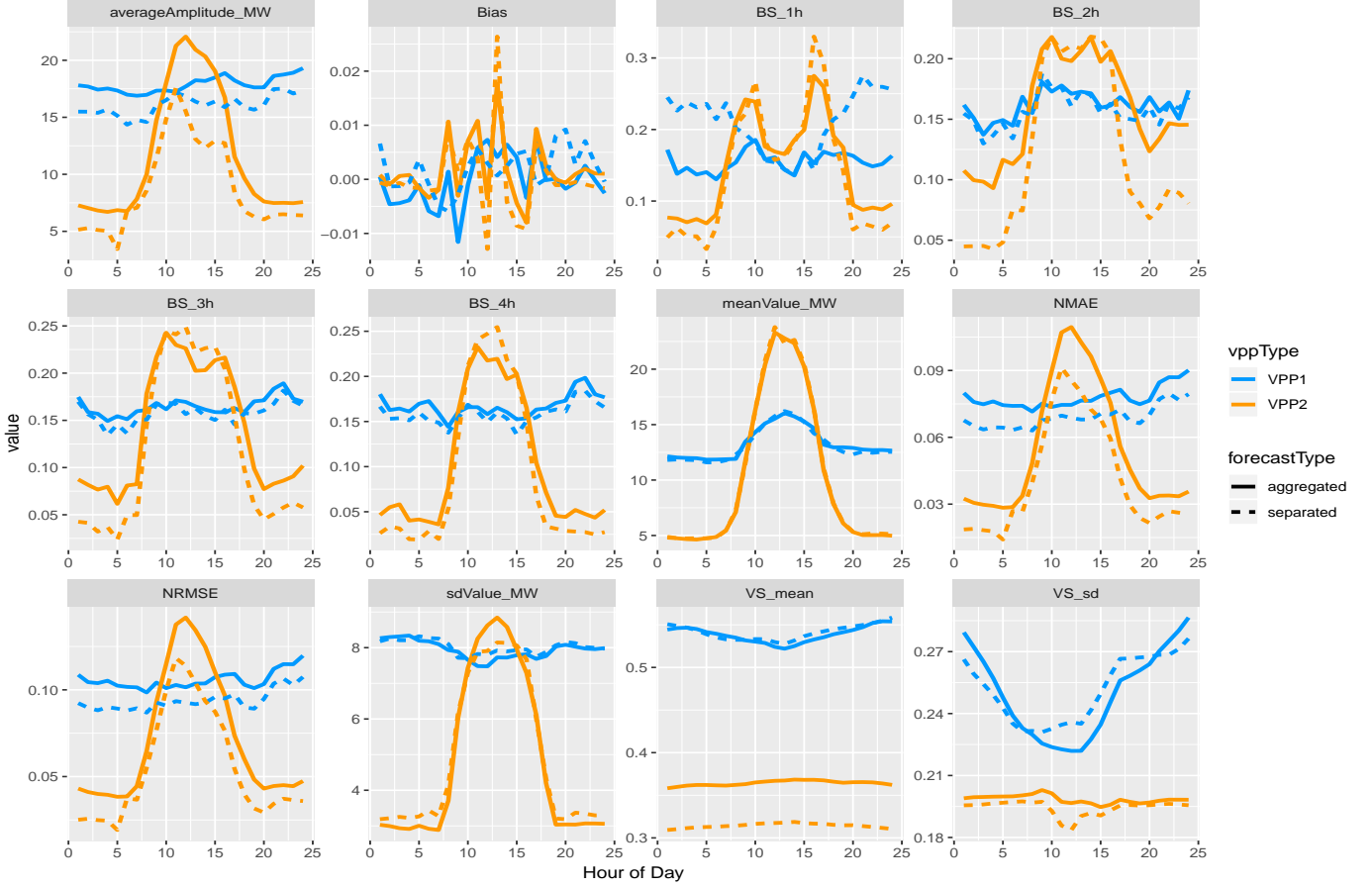
Figure 5: Properties and scores of scenarios generated with Gaussian Copula, directly aggregated from the DG method ("aggregated", solid line) and indirectly aggregated by separate production forecast from the IG method ("separated", dashed-line). Starting at top-left: average Amplitude of the scenario set, in MW; average bias of scenarios, scaled by installed capacity; Brier Score for ramps on several intervals, from 1 hour to 4 hours; mean value of scenarios, in MW; Normalized Mean Average Error of scenarios (NMAE), scaled by installed capacity; Normalized Root Mean Square Error of scenarios (NRMSE), scaled by installed capacity; standard deviation of the scenarios, in MW; mean value of the Variogram Score with moment = 0.5; standard deviation of the Variogram Score with moment = 0.5
