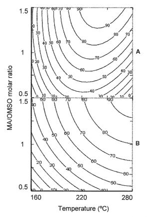
**FIG. 2.** Predicted contour levels for (A) the yield (molar%) of ASA from methyl oleate and (B) the conversion (wt%) of methyl oleate as a function of temperature and MA/OMSO molar ratio. For abbreviations see Figure 1.
