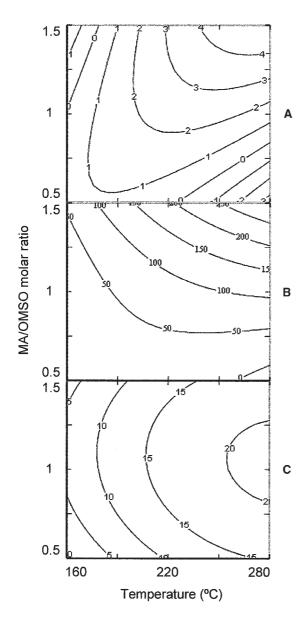
**FIG. 3.** Predicted contour levels for (A) the formation of side products (wt%), (B) the viscosity (cP), and (C) the Gardner color as a function of temperature and MA/OMSO molar ratio. For abbreviations see Figure 1.
