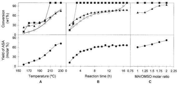
**FIG. 1.** Evolution of the conversion of various reagents and the yield of alkenyl succinic anhydrides (ASA) from methyl oleate as a function of temperature, reaction time, and maleic anhydride/oleic motif-enriched sunflower oil methyl ester (MA/OMSO) molar ratio (■: methyl linoleate, ▲: methyl oleate, ∮maleic anhydride, ●: ASA from methyl oleate).
