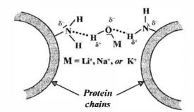
Figure 4. Schematic representation of noncovalent interaction forces between protein chains and ionic bases.
