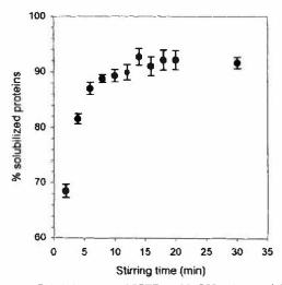
**Figure 1.** Solubilization of ISFP in NaOH solution (pH 12) as a function of the stirring time of 20 mL of film formation solution in a homogenizer (19000 rpm). Average and standard deviation values of three experiments were plotted.
