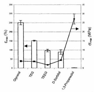
**Figure 5.** Effect of plasticizer type on tensile strength ( $\sigma_{max}$ ) and elongation at break ( $\epsilon_{max}$ ) of ISFP films. Plasticizer/ISFP = 0.00545 mol/g. Average and standard deviation values of five experiments were plotted.
