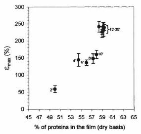
**Figure 2.** Variation of elongation at break ( $\epsilon_{max}$ ) as a function of protein content in ISFP films obtained by variation of the stirring time [numbers next to points correspond to stirring times (minutes)]. Average and standard deviation values of five experiments were plotted.
