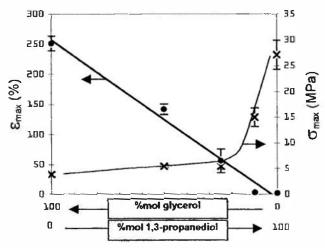
**Figure 6.** Mechanical properties of ISFP films cast with mixtures of glycerol and 1,3-propanediol. Total plasticizer/ISFP = 0.00545 mol/g. Average and standard deviation values of five experiments were plotted.
