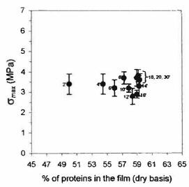
**Figure 3.** Variation of tensile strength ( $\sigma_{max}$ ) as a function of protein content in ISFP films obtained by variation of the stirring time [numbers next to points correspond to stirring times (minutes)]. Average and standard deviation values of five experiments were plotted.
